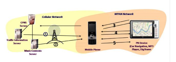
Figure 2: High level diagram showing the flow between cellular network and WPAN using multiple channels
