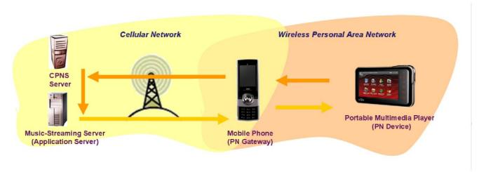
Figure 3: High level diagram showing the flow for contents delivery between cellular network and WPAN
