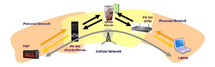
Figure 8: High level diagram showing Remote PNE connection
