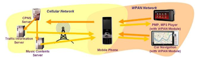
Figure 4: High level diagram showing the flow for simultaneous multiple Services between cellular network and WPAN
