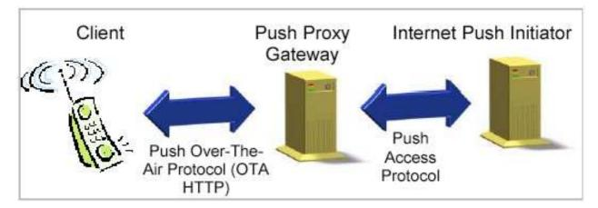
The model is analogous to the push model described in [SYNCWSP] with the difference being that instead of the push services between the Push Proxy Gateway (PPG) and the device being defined by the OTA-WSP protocol they are defined by the OTA-HTTP protocol. Full details of the specifics of both of these are described in [PUSH].
