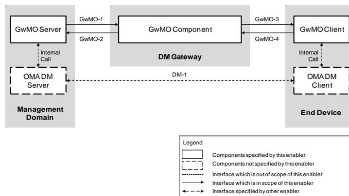
Figure 1: Transparent Mode GwMO Architectural Diagram Using Interfaces
