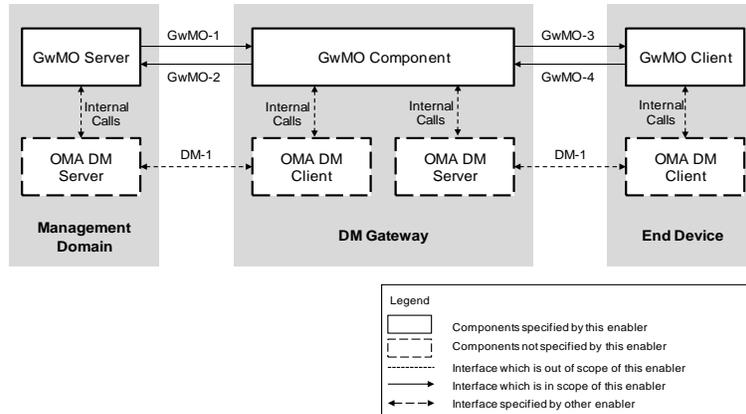
Figure 2: Proxy Mode GwMO Architectural Diagram Using Interfaces
