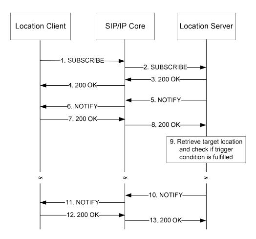
Figure 4: Flow for Subscribing to the Notification of Area Event Trigger
