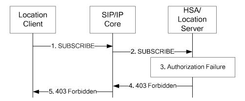
Figure 6: Flow for Subscription Authorization Failure
