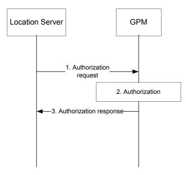
Figure 11: Flow for permissions checking with GPM
