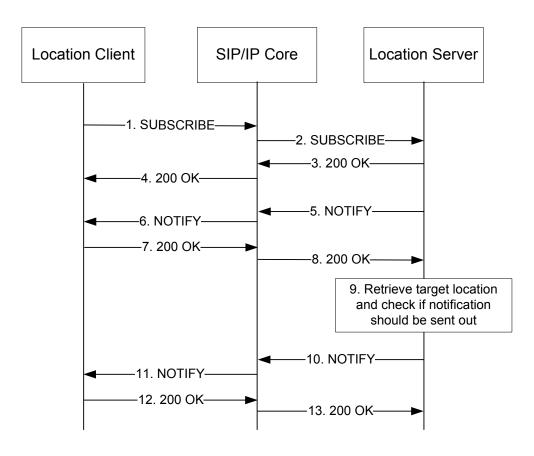
Figure 3: Flow for Subscribing to the Notification of Periodic Trigger
