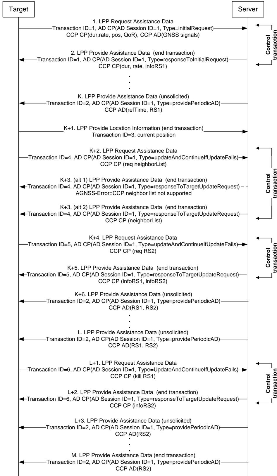
**Figure 21: CCP assistance data transfer – change of reference station**
