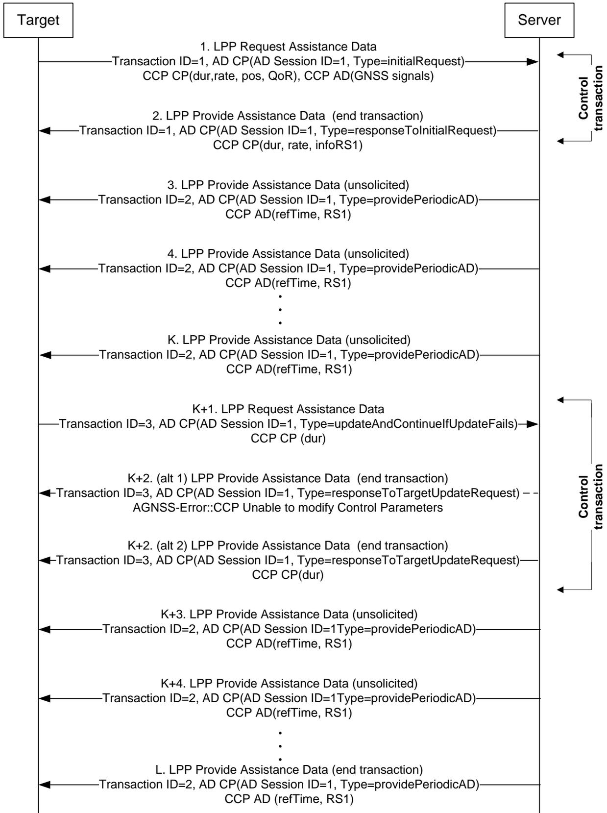
Figure 19: CCP assistance data transfer – session parameter modification (target)
