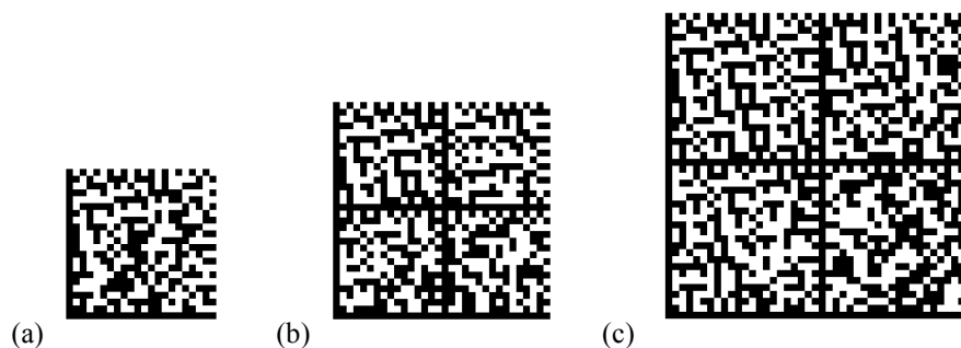
Figure 3. Data Matrix codes encoding alphanumeric data “a123456789a12...” of length (a) 40, (b) 100, (c) 200 characters.
