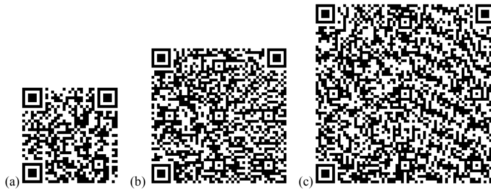
Figure 2. QR codes encoding alphanumeric data “a123456789a12...” of length (a) 40, (b) 100, (c) 200 characters
