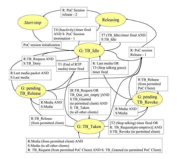
NOTE: T1 is the 'End of RTP Media' timer, T2 is the 'Stop talking' timer, T3 is the 'Stop talking grace' timer, T4 is the 'Inactivity' timer and T7 is the 'Talk Burst Idle' timer.
