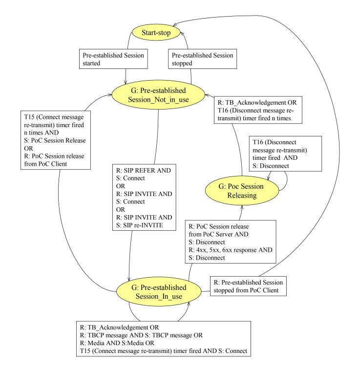
NOTE: T15 is the 'Connect message re-transmit' timer and T 16 is the 'Disconnect message re-transmit' timer.
