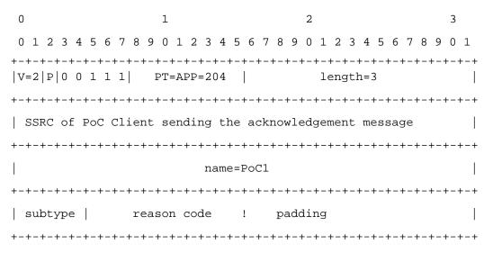
The following bit pattern in the subtype field SHALL be used for the TBCP Talk Burst Acknowledgement message: 00111.
