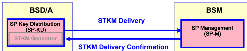
Figure 27 – Alternative Message Flow between BSM and BSD/A for Delivery STKMs
