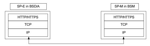
Figure 15 – Protocol Stack for SP-4-1
