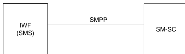
Figure 1 CPM - SMS interworking architecture
