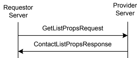
Figure 49: The “ GetListProperties ” Transaction
