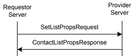
Figure 50: The “SetListProperties” Transaction
