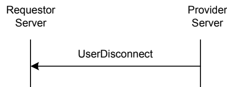
Figure 24. The “UserDisconnect” Transaction
