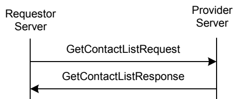
Figure 45: The “GetContactList” Transaction
