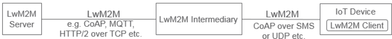
Figure 7 : E2E Security with Intermediate Nodes
