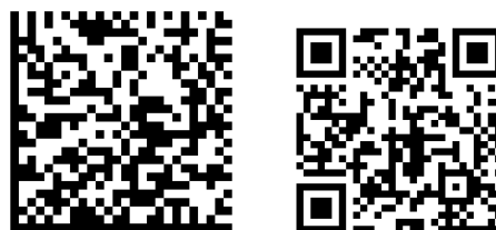
Figure 5. Link to www.openmobilealliance.org encoded as a Smart Poster record (and as Data Matrix and QR)
