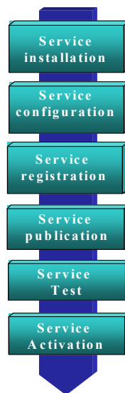
Figure 2– Service Deployment Steps
