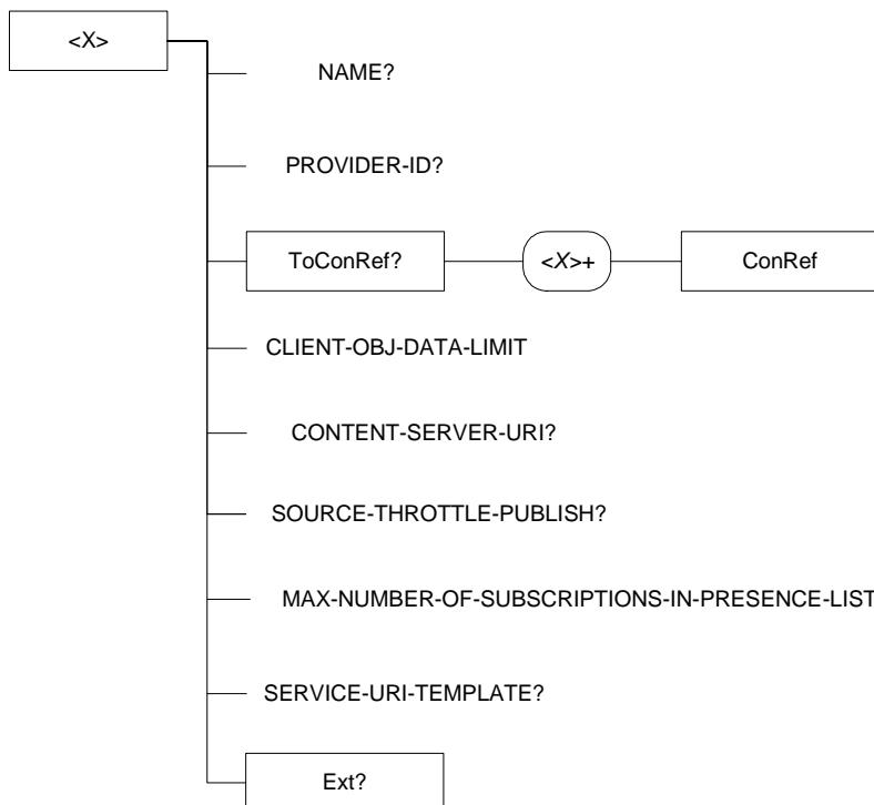
**Figure 1: The OMA Presence SIMPLE Management Object tree**
