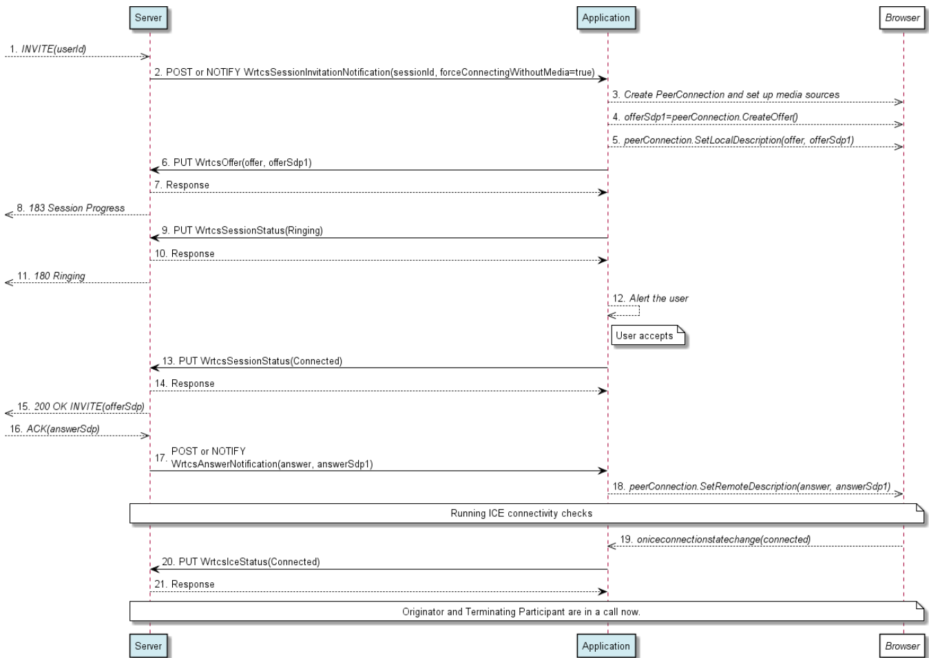
Figure 24: Handling of offerless invitations if reliable provisional responses are not supported
