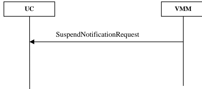
Figure 24: Flow of Suspension Notification Registration Message Exchange
