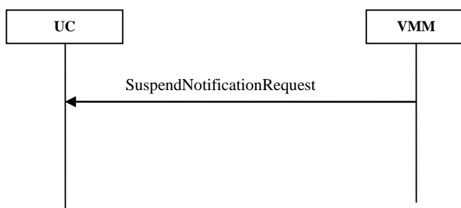
Figure 24: Flow of Suspension Notification Registration Message Exchange
