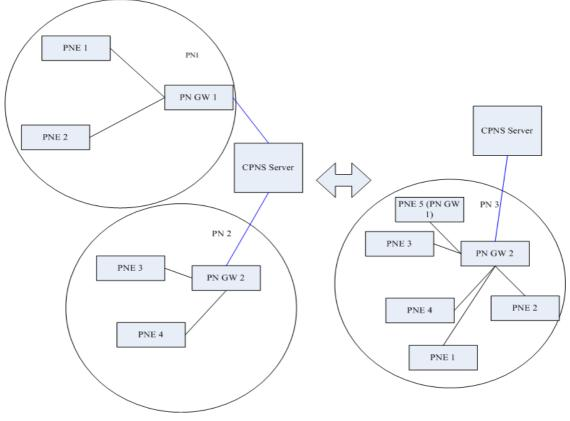
Figure 2. Merging and Splitting of PNs
