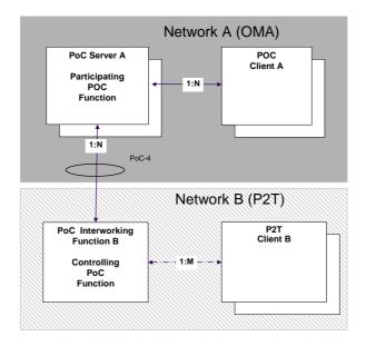
Figure 2: Usage scenario 2 with PoC Interworking Function performing the Controlling PoC Function.
