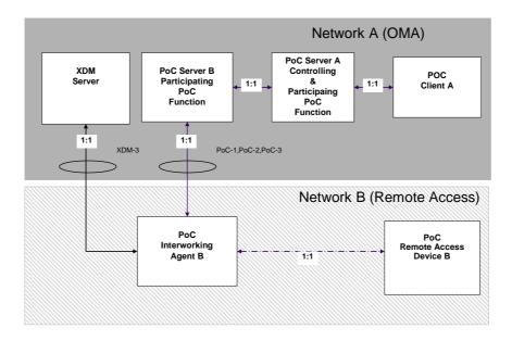
Figure 3: Usage scenario 3 with PoC Interworking Agent supporting PoC Remote Access.
