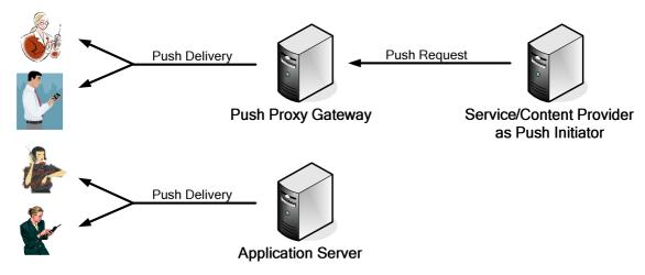
Figure 2: OMA Push service environment with PTM-Push support
