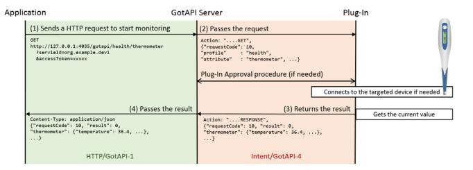
Figure 6: Message flow of the One-shot measuring API
