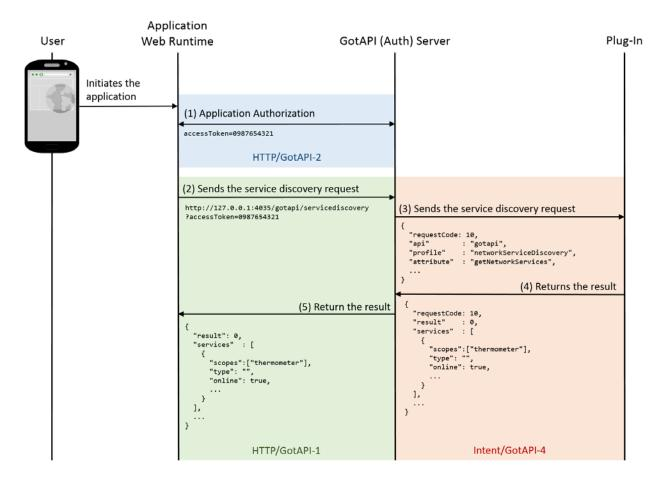
Figure 5: Message flow of the Service Discovery: Message flow of the Service Discovery
