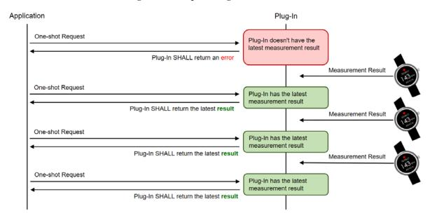
Figure 9: Example of continuous measurement.
