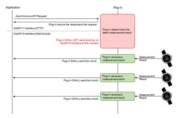
Figure 10: Example of asynchronous messages (continuous measurement).
