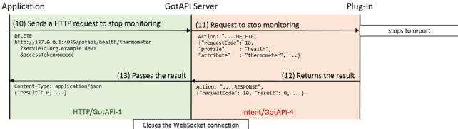
Figure 7: Message Flow of the Asynchronous messaging API
