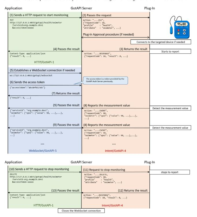
Figure 3: Message Flow of the Asynchronous messaging API
