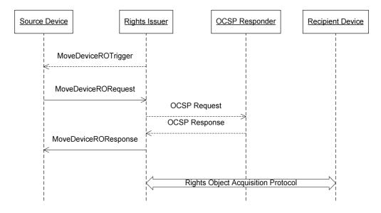
Figure 1 the 2-pass Move Device RO Protocol
