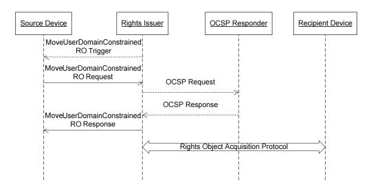
Figure 2 the 2-pass Move <userDomain>-constrained RO Protocol
