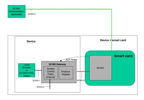
Figure 1: SCWS Connectivity Architectural Model
